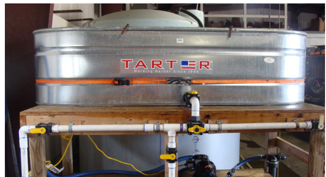
TOP AND LEFT: Commercially available brine production systems. Commercial systems come in a variety of sizes from a variety of manufacturers and brine production rates vary based on the specific unit. The units pictured can produce brine at rates of 1,000 gallons an hour up to 6,000 gallons an hour.
