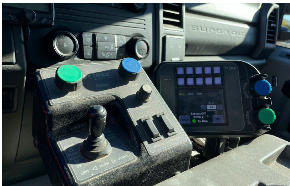
In cab controls for ground speed-controlled spreader.
