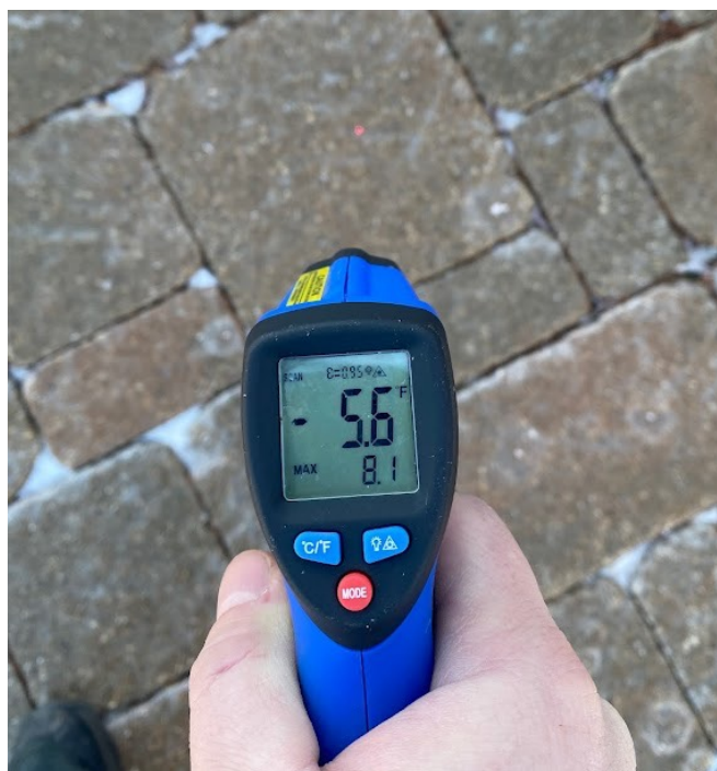
Hand-held infrared temperature sensor.
