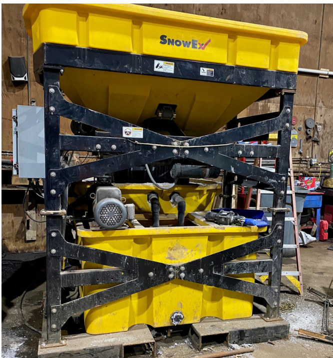
TOP AND LEFT: Commercially available brine production systems. Commercial systems come in a variety of sizes from a variety of manufacturers and brine production rates vary based on the specific unit. The units pictured can produce brine at rates of 1,000 gallons an hour up to 6,000 gallons an hour.
