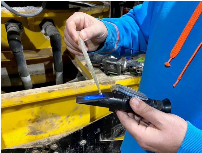
Measuring the salt brine concentration with a refractometer. A sample of brine is placed on the plate and the concentration is read through the eyepiece at the other end.
