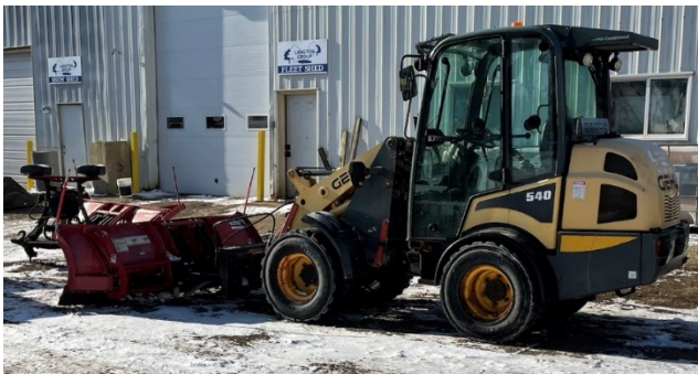
Right and Above: Plows and snow pushers can be mounted to small loaders or skid steers for use in parking lots and tight spaces.
