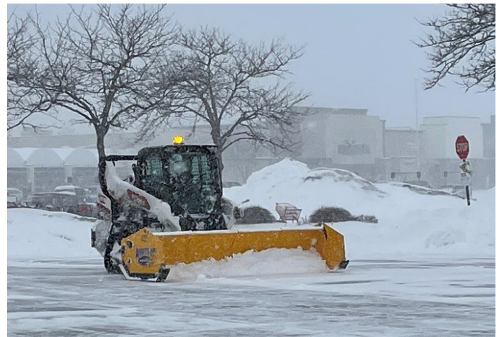
Right and Above: Plows and snow pushers can be mounted to small loaders or skid steers for use in parking lots and tight spaces.
